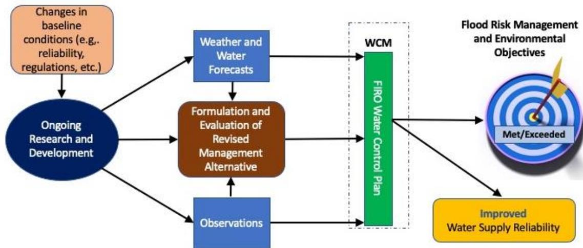
**Figure 6.6.** Conceptual framework for a FIRO WCP that effectively adapts to (1) changes in baseline conditions, (2) weather and water forecast skill, (3) improved observations, and (4) improved reservoir management models.
