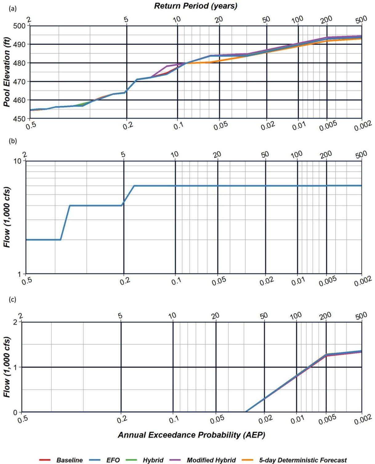
**Figure 3.16.** Annual maximum (a) pool elevation, (b) total release, and (c) uncontrolled spill frequency functions at Lake Sonoma. Results for all alternatives are nearly identical in the bottom two plots.
