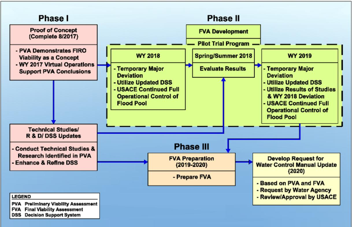
**Figure 1.1.** The initial process diagram and timeline for the FIRO program at Lake Mendocino, consisting of three phases for moving from the PVA to the request for a change to the WCM. Note that Phase II was delayed one year from the initial plan. This FVA document is represented by the beige box under Phase III. It will be followed by a request for an update to the WCM.
