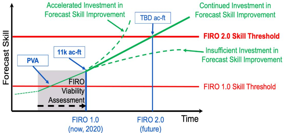
**Figure 1.12.** The FVA concludes that current forecast skill is sufficient to support using forecasts in Lake Mendocino operations, yielding up to roughly 11,000 ac-ft of additional water supply reliability or flood mitigation capacity. This figure illustrates how future improvements in forecast skill could enable even greater flexibility in operating the reservoir, and how achieving this is supported by research to improve predictions of ARs and their associated precipitation and runoff.
