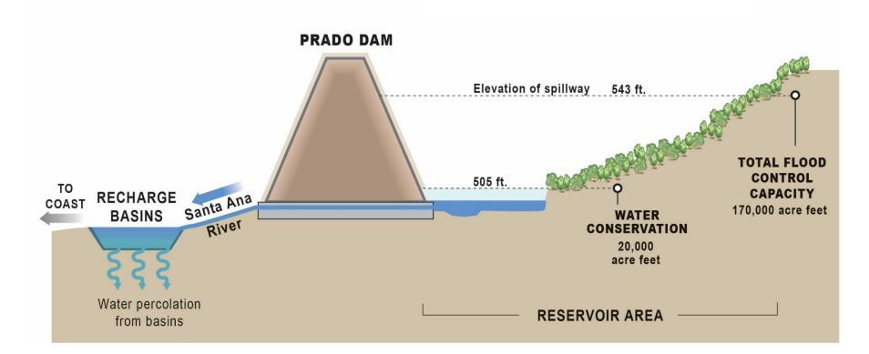
Water held below elevation 505 ft is released at rate OCWD can recharge it downstream
