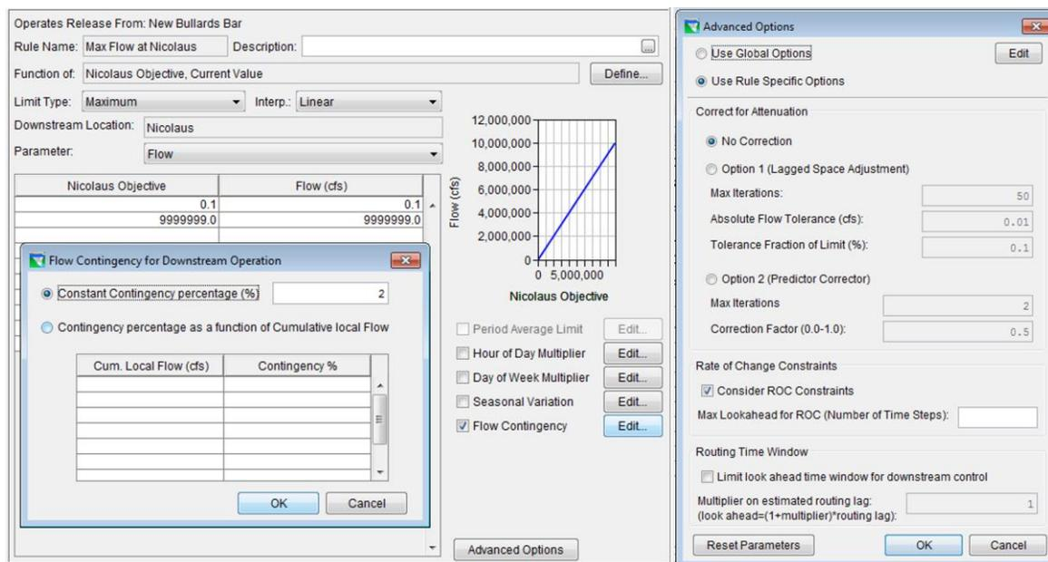
**Figure 3-19.** HEC-ResSim downstream control flow rule: max flow at Nicolaus with advanced flow contingency options.
