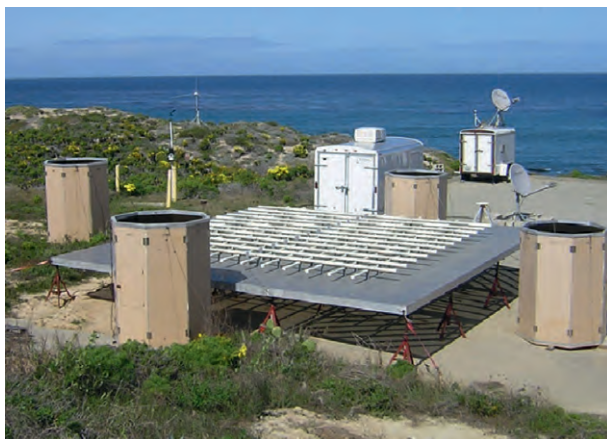
FIG. 8. The ARO installed on San Nicolas Island off the coast of Southern California. The gray panel in the middle of the photo is the frame for the 449-MHz wind profiler coaxial-colinear phased array radar antenna. The octagonal enclosures house the acoustic antennas that are part of the RASS for temperature profiling. The wind profiler and RASS electronics are situated in the environmentally controlled trailer. The site also includes a 10-m meteorological tower (not shown) and a GPS receiver for IWV estimates.
