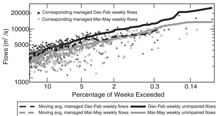
**Fig. 10** Estimated exceedence probabilities (*solid curves*) of unmanaged 7-day average outflows from the Central Valley, above the Sacramento-San Joaquin Delta, in winters and springs, 1967–1987, with corresponding managed-flow estimates as *circles*, as based on time series from Knowles, 2002. *Dashed curves* are moving averages of circles, showing the 20-episode average managed flows around each level of unmanaged flow rate
