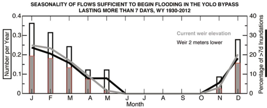
**Fig. 9** Numbers (bars) and fractions (curves) of occasions when Sacramento River flows at Verona (USGS gage #11425500) were sufficient for overtopping the Fremont Weir that controls inundations of the Yolo Bypass floodplain, with the existing weir (grays) and for a hypothetical case of a weir height 2 m lower (black), from October 1929 through September 2012
