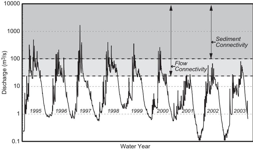
**Fig. 6** Hydrograph from 1995 through 2003 showing thresholds for flow and sediment connectivity. Channel-floodplain flow connectivity occurred in all years, but sediment connectivity only occurred during 1995–2000. Adapted from Florsheim et al. 2006
