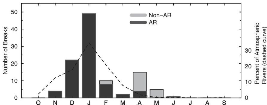
**Fig. 4** Seasonality of 109 well-reported levee breaks on Central Valley rivers between 1951 and 2006, with indication of whether or not each levee break coincided with an atmospheric-river storm; *dashed curve* indicates average monthly frequencies (seasonality) of occurrence of all landfalling ARs in California (from Table 2, Dettinger et al. 2011)
