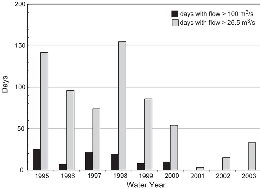
**Fig. 7** The number of days when flow ( $Q$ ) exceeded thresholds for hydrologic connectivity ( $Q/Q_c > 1$  corresponding to 25.5 m³/s) and sediment connectivity ( $Q/Q_c > 4$  corresponding to 100 m³/s) illustrated after intentional levee break for years between 1995 and 2003. Adapted from: Florsheim et al. 2006
