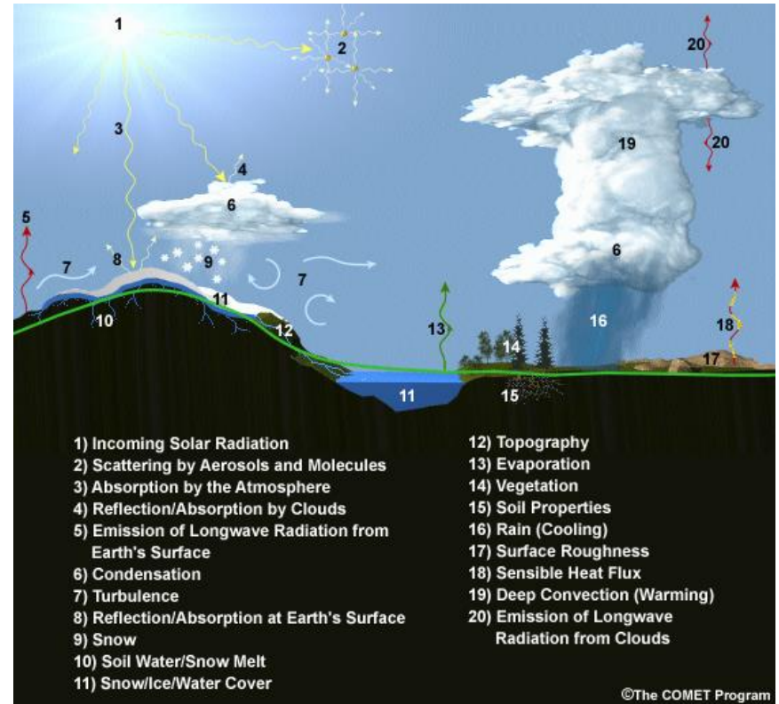
Processes and physical model elements that are represented in NWP models
