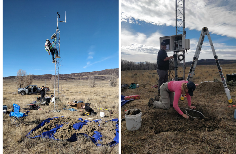
Team members work to install the meteorological sensors on the Howe Ranch Station tower in the Upper Yampa River Basin in Colorado with soil from the soil pit laid out in the foreground.
