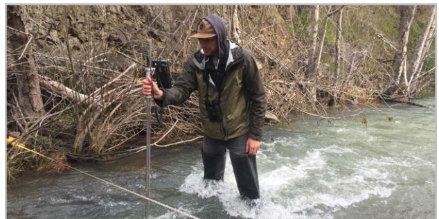
A CW3E researcher measuring streamflow at a site in the upper Russian River watershed in March 2018.
