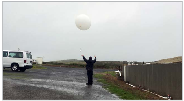
A CW3E researcher releases a radiosonde during a January 2017 AR at the UC Davis Bodega Marine Lab in the Russian River watershed.
